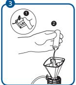
MONOMER FILLING Start the vacuum pump. Fill the monomer.
