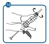
DISPENSING – ENGAGE While holding the unit, rotate cylinder to a full stop.
